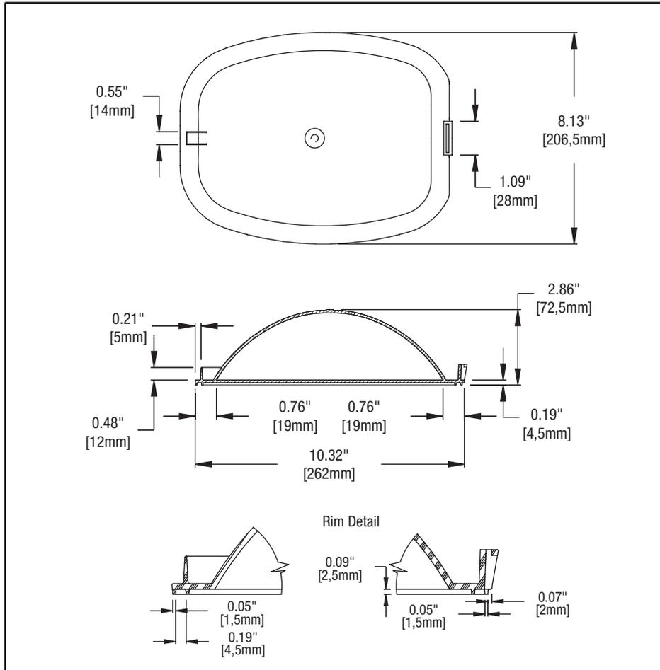
**This drawing is for reference only. Actual part dimensions will vary. Customer is urged to review actual samples to confirm fit and function. All specifications and dimensions are subject to change without notice.**
